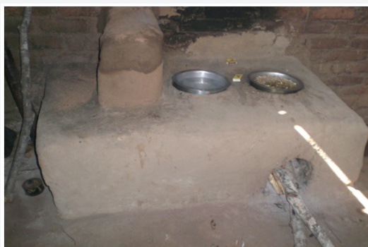
Plate 6: With ICS, smoke and dust are fully controlled and directed outside the kitchen environment through the chimney
